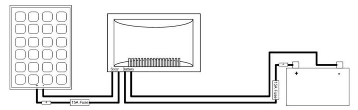
1. Connect the "Solar" lead to the Solar Panel like shown in the diagram above.
